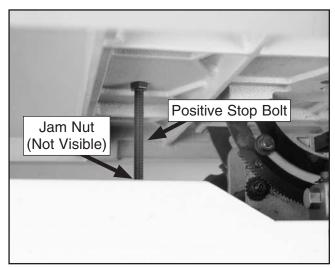
Figure 19. Positive stop bolt and jam nut.
